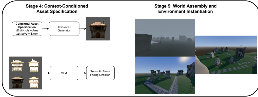
Figure 2: Context-conditioned asset grounding and world assembly. Given the resolved tile-based world layout, context-conditioned 3D assets are generated for each entity by conditioning text-to-3D prompts on the entity’s semantic role, local area narrative, and global style constraints (Stage 4). Because text-to-3D models produce meshes with arbitrary orientation, canonical front, back, left, and right views are rendered and a vision-language model is used to identify the semantic front-facing direction when required. The resolved tile-based layout and oriented assets are then deterministically assembled into an executable environment instantiated in the Godot engine, producing a coherent and traversable 3D world (Stage 5).
